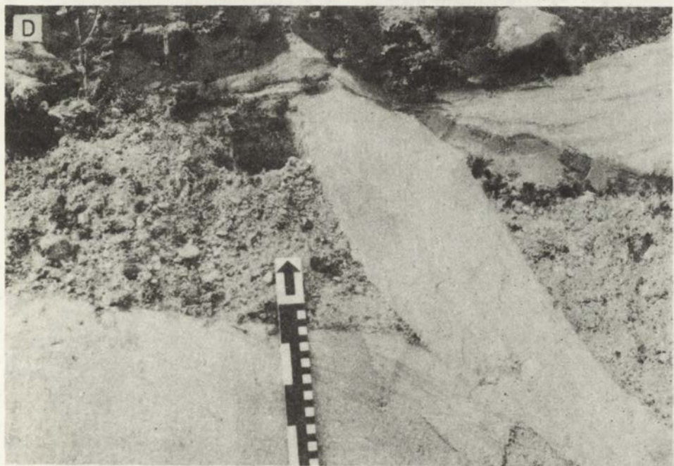
Structure of basal lodgement till in tunnel valley slope pit (the Leszno-Osieczna case study area)
