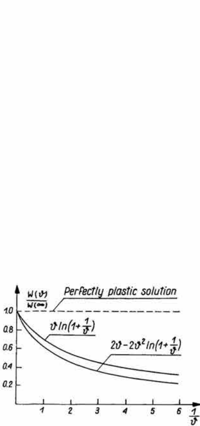
FIG. 9. Reduction of response time and permanent deflections of a rectangular plate due to viscosity of the material.
