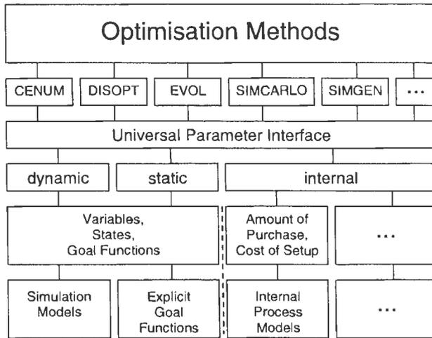
**Figure 3.** The *ISSOP* optimisation architecture
