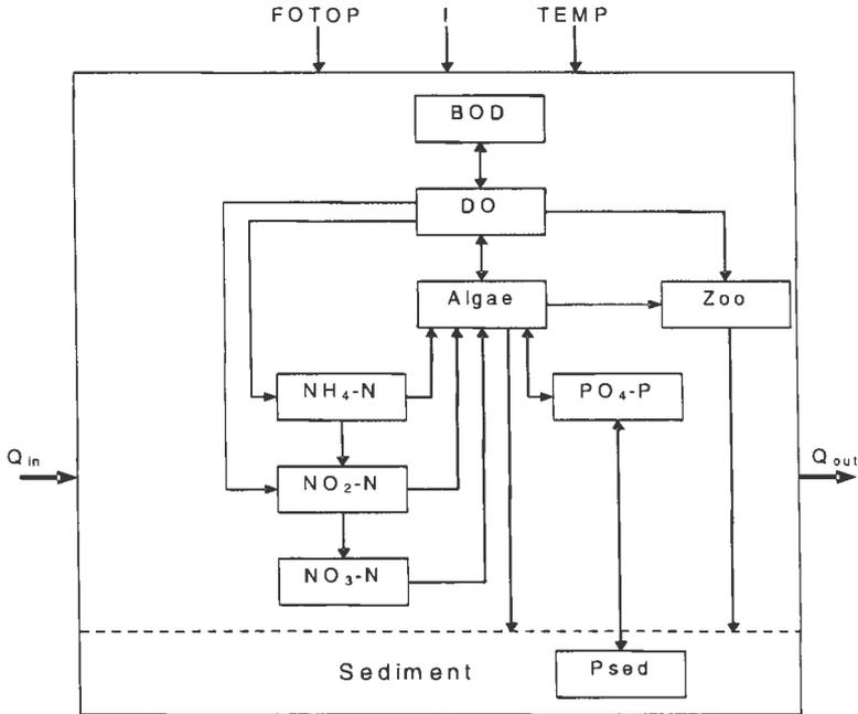
**Figure 2.** Conceptual model of the eutrophication simulator
