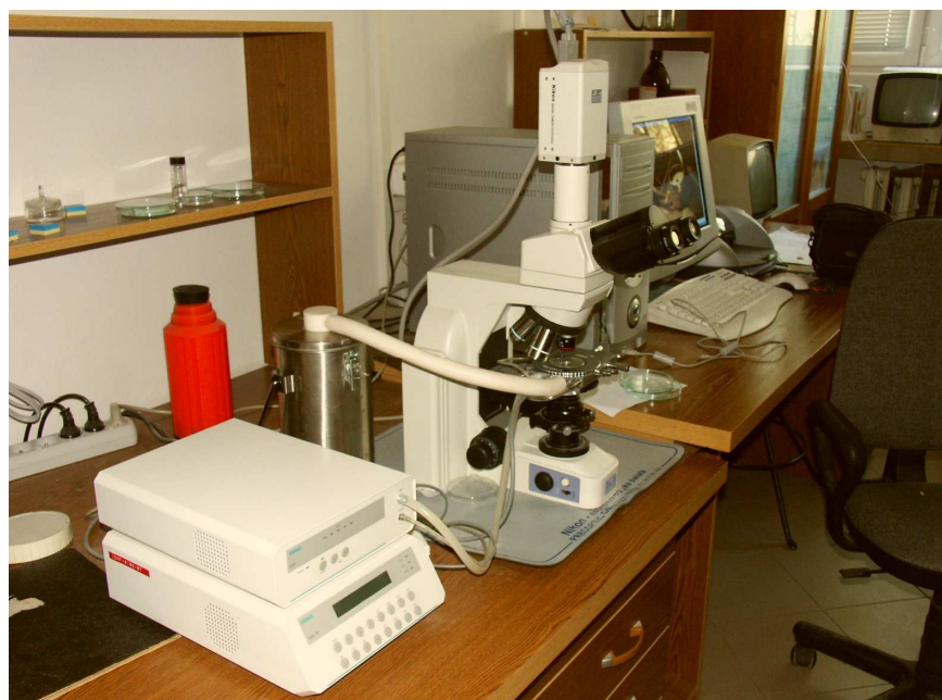
Figure 58. The optical polarizing microscope Nikon ECLIPSE E 400 equipped with Nikon Digital Camera DXM 1200 and a heating/cooling stage LINKAM THMS 600 with 0.01^\circ control of the temperature.
