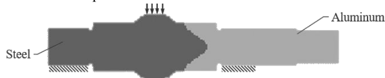
Figure 3: Optimized result for the hybrid shaft under bending with IZEO and manufacturing constraints.
