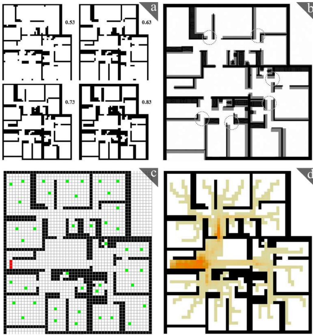
Figure 4: a). Different binarization thresholds produce layouts of substantially different resemblance to the original. b). The binarization at 0.73 threshold compared to the original layout (shown in black in the background). Since the grid is very coarse, certain openings and corridors become too narrow, as indicated by the dotted circles. d). Manually corrected layout, so the widths of the corridors and openings are proper. The positions of exits and agents are shown in red and green, respectively. e). The heat map shows that although the exit area is perhaps a little narrow, the layout is rather safe.
