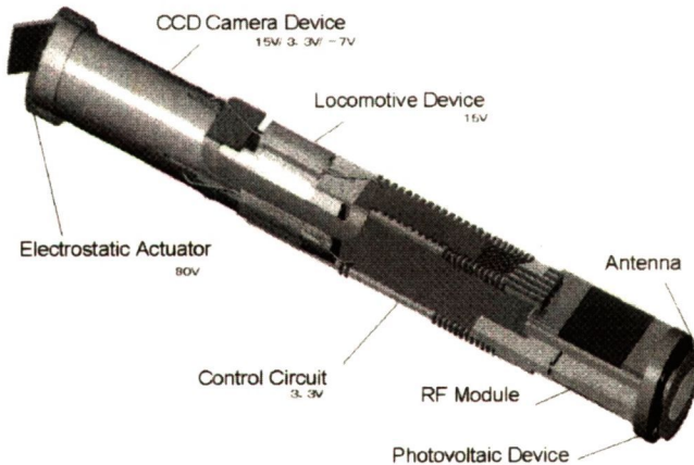
Fig.1. System image of wireless micromachine for inspection on inner surface of tubes.
