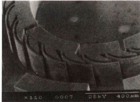
Fig.7. SEM image of the cantilever terminals.
