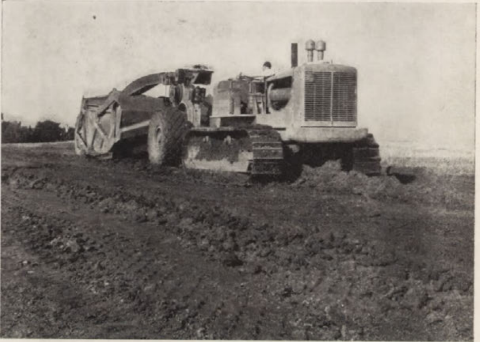
Fig. 3. Mechanical scraper drawn by diesel-engined tractor Used in opencast quarrying for removing soil, and for levelling and soil replacement
