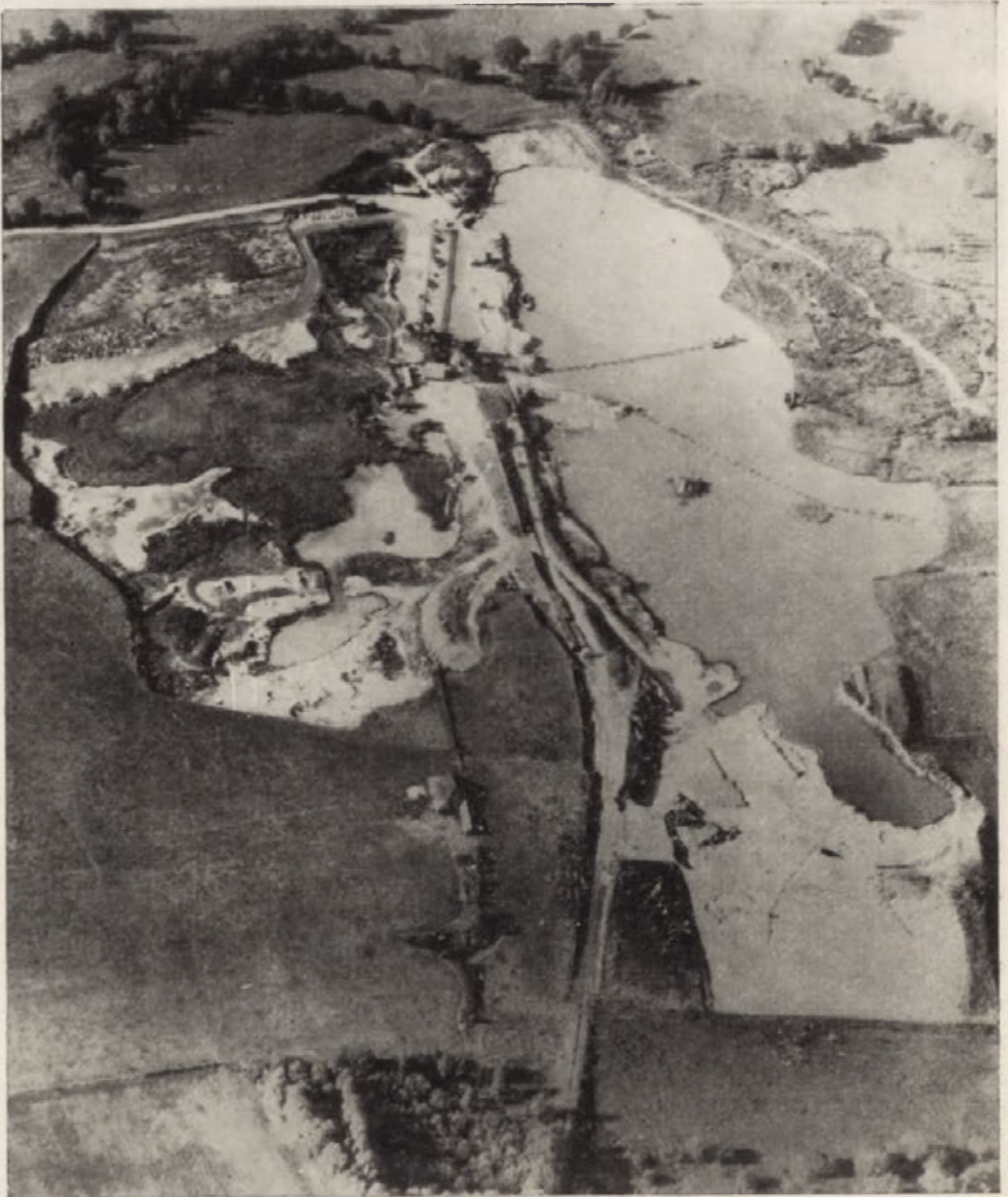
Fig. 8. Aerial view of a "wet" gravel pit ("Type 4") in North Kent Gravel dredged from lake-bottom. Bottom right, soil stripped from gravel bed; centre left, filling in progress; top left, filling complete, soil being replaced
