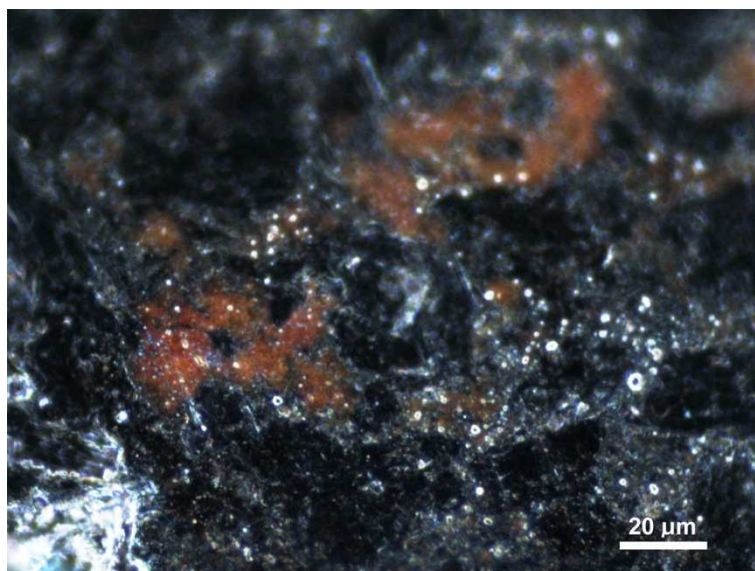
Fig. 13.1. Optical micrograph of syringaldazine modified CCE surface. Red islands correspond to syringaldazine deposit.
