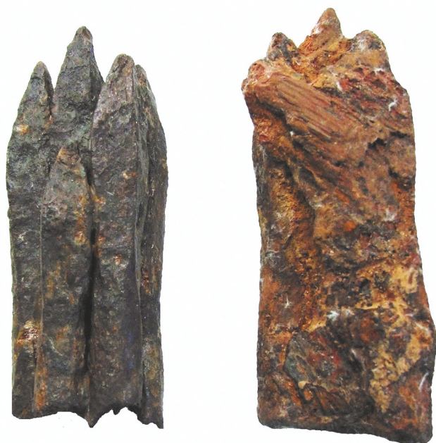
Fig. 9. Five boltheads melted together during a fire. Vassal House in Křivoklát Castle. Photo J. Hložek.
