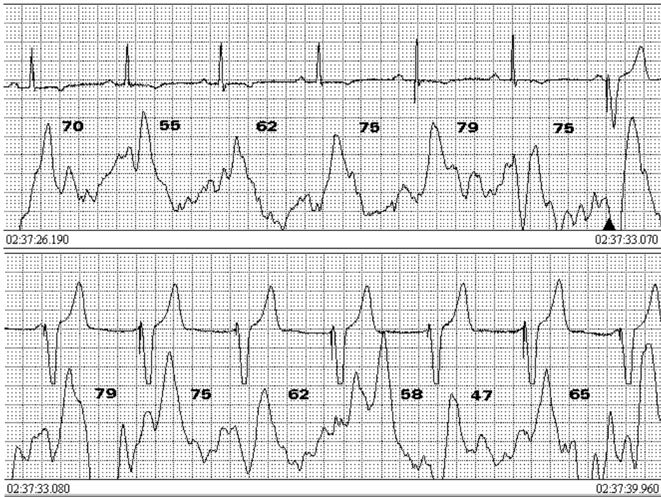
Figure 5.9. The simultaneous recordings of one ECG channel and the impedance cardiography first derivative signal ( dz/dt ) in the patient with pacemaker. The top strip contains traces recorded during normal sinus rhythm (SR) and the bottom strip shows signals recorded when pacemaker syndrome occurred (3 rd , 4 th , and 5 th cycle). The numbers at the impedance trace denote stroke volume expressed in ml.
