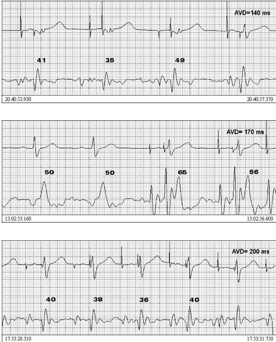
Figure 5.8. Optimisation of atrio-ventricular delay (AVD) in patients with dual-chamber pacemakers using ReoMonitor. Excessively short (top) and excessively long (bottom) AVD result in decreased stroke volume (given in ml). The optimal AVD = 170 ms (middle strip) was selected when stroke volume was maximal.
