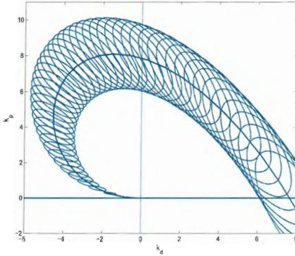
Fig. 4. Ellipses corresponding to  $\delta = 0.2$  with  $\mu = 0.5$  and  $\omega \in (0.001, 2.4)$  rad/s.
