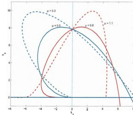
Fig. 2. Stability regions for different values of the exponent  $\mu$  of the derivative term (regions below the curves corresponding to each value of  $\mu$  and above the horizontal axis).
