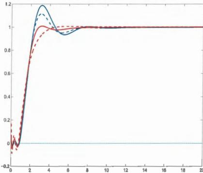
Fig. 5. Step responses of the feedback control system for  $k_p = 3.0$  and  $k_d = 1$  with  $\mu = 0.3$  (solid blue),  $\mu = 0.5$  (dashed blue),  $\mu = 0.8$  (solid red) and  $\mu = 1.1$  (dashed red).
