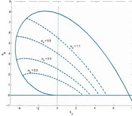
Fig. 3. Loci of constant gain crossover frequency  $\omega_a$  inside the stability region for  $\mu = 0.5$ .
