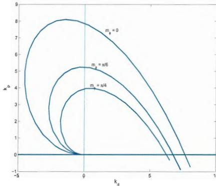
Fig. 1. Locus described by (19) and (20) for  $\mu = 0.5$  and  $m_v = 0$ ,  $m_v = \pi/6$ ,  $m_v = \pi/4$  when the plant transfer function is given by (43). The stability region lies between the curve for  $m_v = 0$  and the  $k_d$ -axis ( $k_p = 0$ ).
