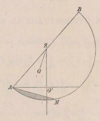
segment AM ( $\angle SAM = \beta$ ) made solid. G in the line SG at right angles to AM is the c.g. of the lamp, and G' the c.g. of the oil.
