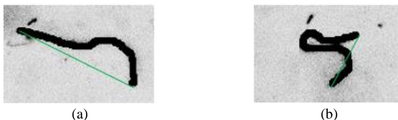
Figure 4.7. End-to-end distance, example of EE evaluation: (a) EE = 0.84 ; (b) EE = 0.38 .
