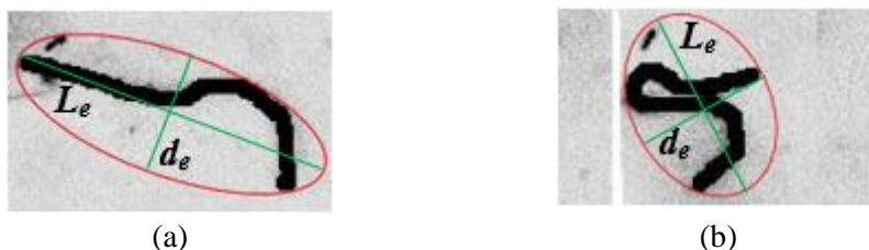
Figure 4.5. Degree of elongation, example of EL evaluation: (a) EL = 0.42 ; (b) EL = 0.60 .
