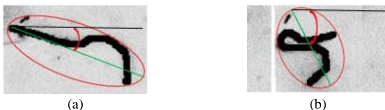
Figure 4.6. Inclination angle, example of IA evaluation: (a) IA = -24.25^\circ ; (b) IA = -73.84^\circ .
