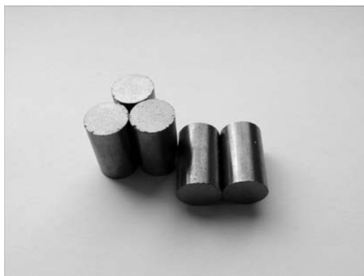
Figure 3.6. Sintered NiAl/Al 2 O 3 specimens.
