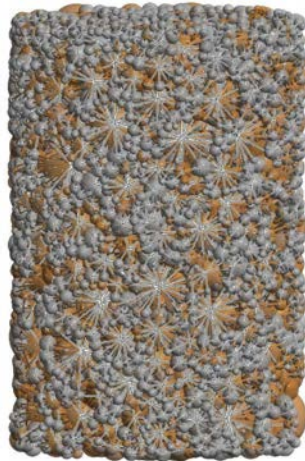
Figure 6.8. Network of particle connections during sintering.
