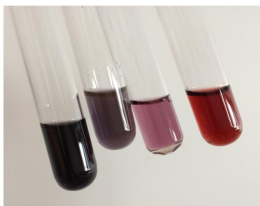
Fig. 1.2. Gold nanoparticles of different diameters obtained by Martin synthesis prepared by the author. The wine color suspension (first from the right) contains the most stable gold nanoparticles of the size of around 3.5 nm.
