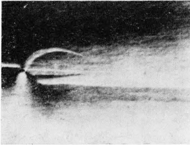
FIG. 1. Plastic zone around the crack tip visualized by etching a steel Fe-3Si specimen [3].
